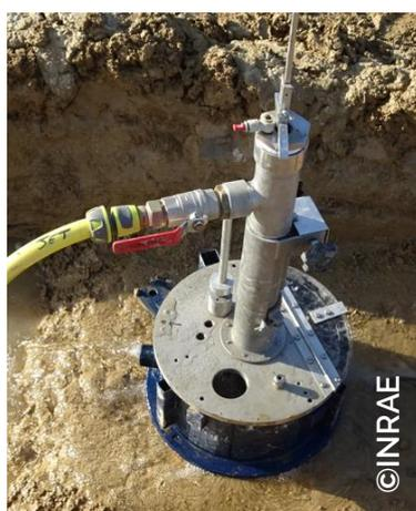
Jet Erosion Test
